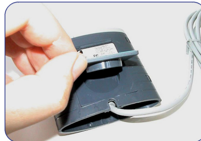
After removing the blue foil, attach the reader to a monitor, etc.
