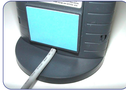
Place the cable in the base cut-out. Tuck the reader using the guide bars into the round opening and press until it snaps.
