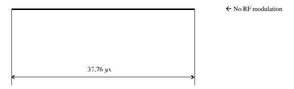
Logic 0 is transmitted by an unmodulated carrier during the whole 37.76 µs bit frame.
