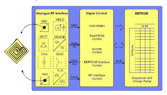
The label requires no internal power supply. Its contactless interface generates the power supply and the system clock via the resonant circuitry by inductive coupling to the read/write device. The RF interface circuitry also demodulates data that are transmitted from the read/write device to the I•CODE Label, and modulates the electromagnetic field for data transmission from the I•CODE Label to the read/write device.
