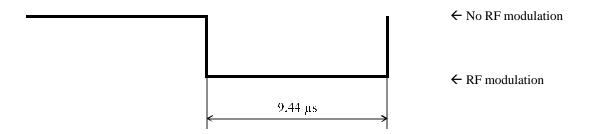
The pulse within one of the 256 bit positions is coded as follows:
