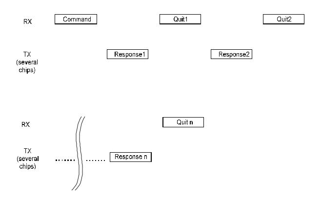
RX .... Command/acknowledgements transmitted from the read/write device to the I•CODE1 Label ICs TX .... Response data transmitted from the I•CODE1 Label ICs to the read/write device
