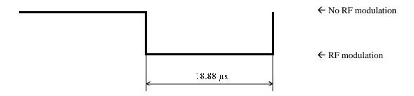
Each byte is started with the LSB, each of the 8 bits within a byte is coded as follows:
