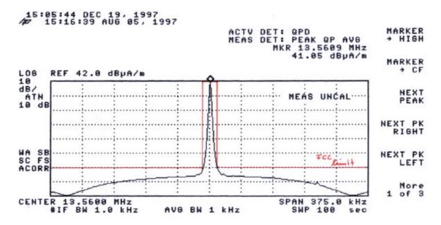
**Note:** The reason for the FCC limit drawn at 60 dB is the used measurement band width of 1 kHz in contrast to 10 kHz, which results in the above mentioned 50 dB side band margin.
